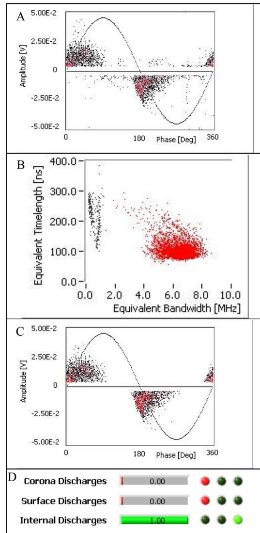
**Figure 5:** Measurement results performed on an online medium voltage cable. A) Entire pattern acquisition; B) Classification map; C) Sub-pattern corresponding to the red cluster on the classification map; D) Output of the automatic identification.
