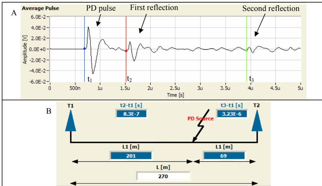
**Figure 6:** Results of the PD localization by the TDR technique, performed on a homogeneous cluster of waveform. A) Average pulse waveform; B) Localization of the PD source.
