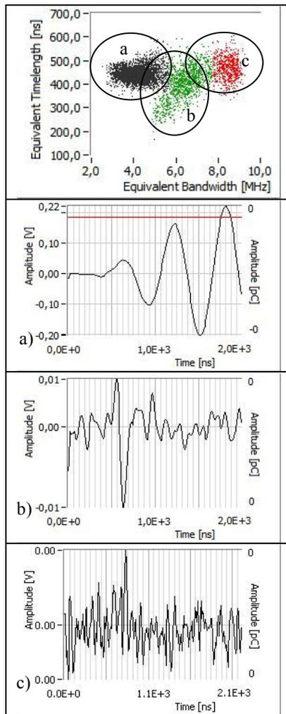
**Figure 1:** Example of feature extraction of different pulses. The differences, in terms of pulse shapes, result in different positioning of the pulses in the equivalent time-length/equivalent bandwidth plane.
