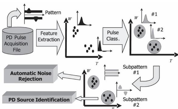
**Figure 2:** PD data processing. Example of two superimposed phenomena consisting of PD activity and noise. Feature extraction and separation (T-W map), pulse classification (Class.), and identification are carried out sequentially.
